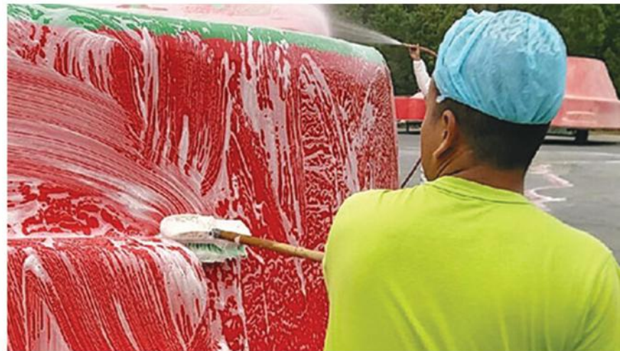
The mold is cleaned and prepared to build your pool on.
